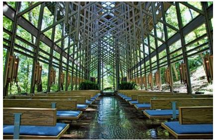
The chapel is made with all organic materials to fit its natural setting. The building materials are primarily pressure-treated pine 2×4s, 2×6s, and 2×12s. The larger elements of the building, such as the trusses, were assembled on the floor and raised into place. Light, shadows, and reflections play a major role in Thorn crown's ambience. Because of the chapel's elaborate trusses and the surrounding trees, constantly changing patterns of
